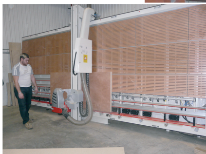
Two Striebig Control vertical panel saws in use at Millennium Door Systems.
