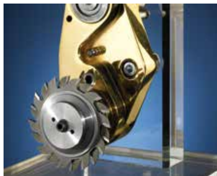
Scoring saw unit VSA with infinitely adjustable saw blade. It safely prevents damage to the edges. It saves time, money and tool costs. If coated panels of a possibly lower quality level are processed, in our opinion, VSA is a "must"!
