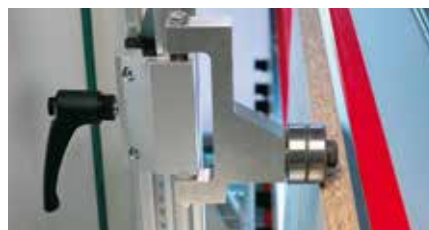
Strip cutting gauge, 400 and 600 mm in length with edge-protecting roller support.
