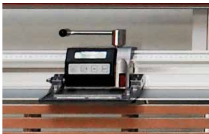
Digital measuring system DMS – for measurements that are accurate to 1/10 mm.
