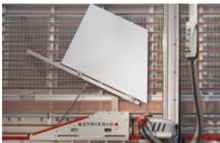
The angle cutting unit WSG maintains the set dimension accurately in all angle settings.
