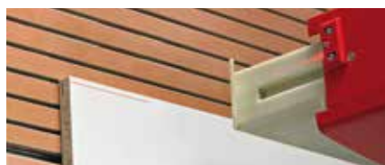
Laser-assisted indication of the horizontal cut (standard)
