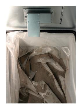
Launched at Ligna, the new contactless AL-KO ALC 21 sensor can be retrofitted onto any Power Unit model. Integrated into a dust-protected sheet steel housing, it has been designed to reliably monitors the level of the chip container via ultrasound and, once it reaches its maximum level, the machine alerts the operator and turns off automatically after 10 minutes if not emptied.
