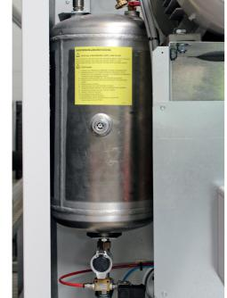
A fire extinguishing system come as standard on larger models (250 and above). The triggering of the extinguishing process is controlled automatically by a temperature sensor via the device controller. Manual
