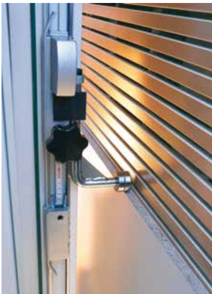
The standard strip cutting gauge with edge-protecting roller support makes repeat cuts easier.
