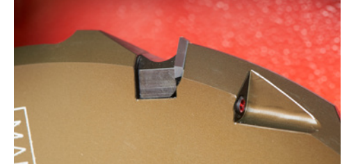
90° grooves (V-shape) for bends up to 90°
