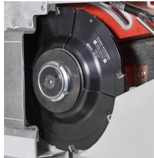
Adjustable grooving tool with reversible carbide tips
