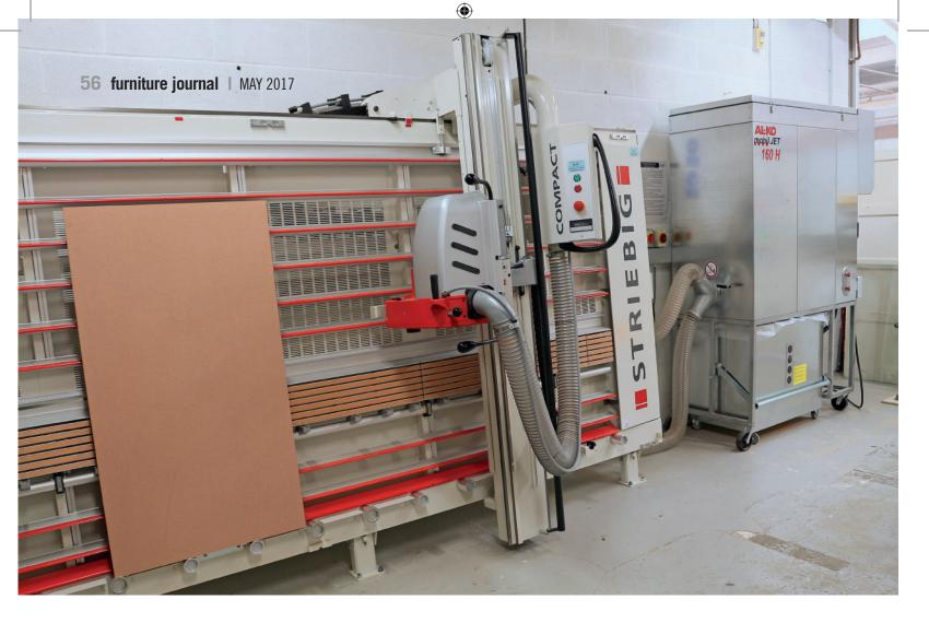
Above: The Striebig compact will cut a wide range of panel materials with precision. All Compact models are also ideally suited for milling and grooving work.
